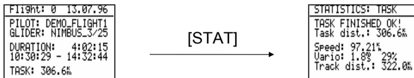
Initially, statistics for the complete task are displayed, showing the length of the declared task, the average speed, portion of vario (flying thermals) and the distance flown. With [VIEW/STAT] again you can see the statistics for the individual legs.
