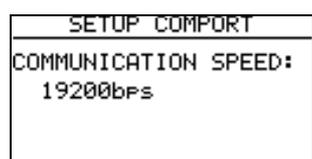
The communication speed is selected with the arrow keys UP/DOWN [^]/[v].
