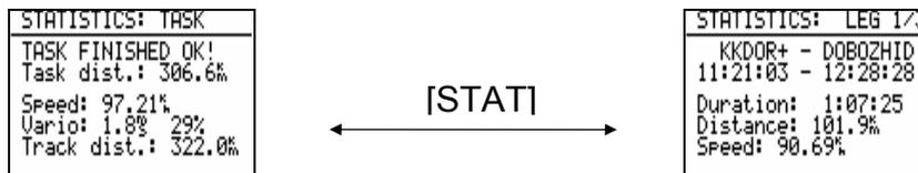
You can select the different legs by using the arrow keys LEFT/RIGHT [<]/[>]. With the UP/DOWN [^]/[v] arrow keys you can switch between the statistic pages of each selected leg.
