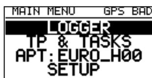
As a first example the logger will be set to a new pilot, a new glider etc (FLIGHT INFO). This will be done in the sub-menu of LOGGER. Choose this sub-menu by moving the cursor to LOGGER using the UP/DOWN [^]/[v] keys and hit [ENTER].
