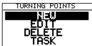
The first three items, NEW, EDIT and DELETE are used for creating, editing and deleting turn points. TASK contains a list of 100 tasks, which can be programmed here.
