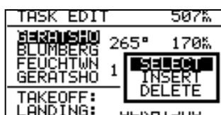
Choose SELECT, enter the first letters of the turn point Erpfting and confirm with [ENTER] or [ESC]. Confirm the suggestion ERPFTING with [ENTER] again and the start point Erpfting will appear as the first point.
