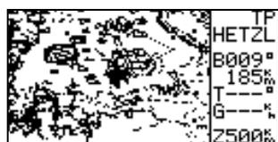
E.g. if one sets the distance value to 50km, the corresponding airspace group will be displayed at a scale of 50km or greater (20km, 10km...). Above that value this airspace will not appear.
